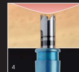
Smart Lift Drill trephine drill digs a core of bone tissue; with an apical-coronal stop at the sinus' cortex
